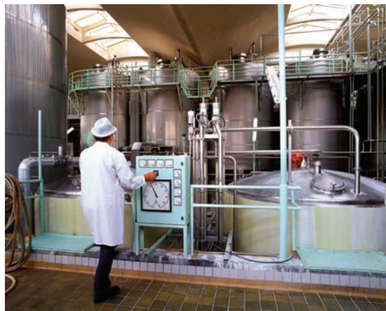
FIGURE 7.7 The Pasteurization of Milk. Milk is pasteurized by passing the liquid through a heat exchanger. The flow rate and temperature are monitored carefully. Following heating, the liquid is rapidly cooled. »» Why is the liquid rapidly cooled?
