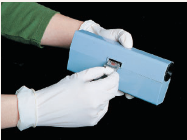
(c) The charged blood chamber is inserted into the slot on the side of the hemoglobinometer.
