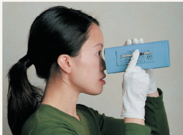
(d) The colors of the green split screen are found by moving the slide with the right index finger. When the two colors match in density, the grams/100 ml and % Hb are read on the scale.
